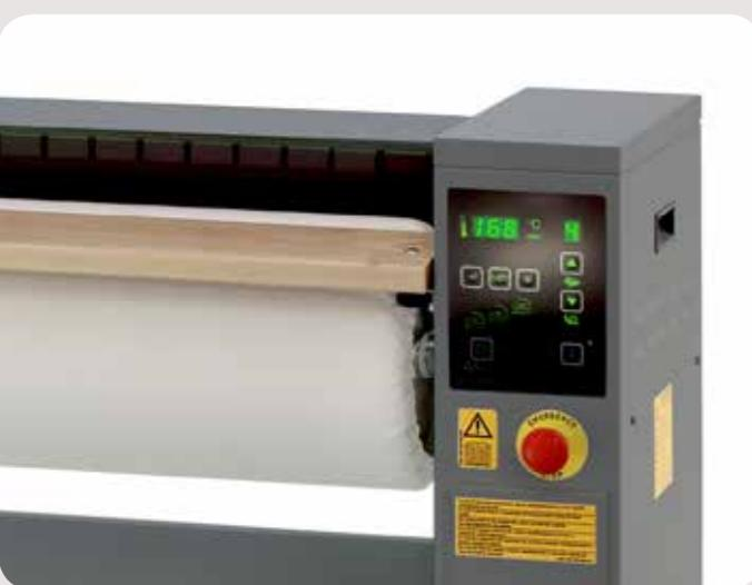
The user electronically selects the desired temperature and adjusts the speed of the cylinder from a control panel.
