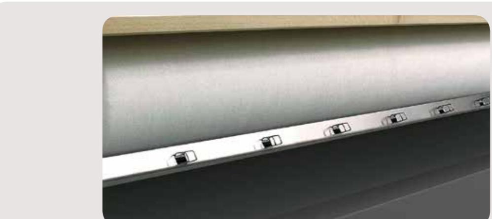
A system of separators placed at the linen outlet prevents the laundry from wrapping around the cylinder.
